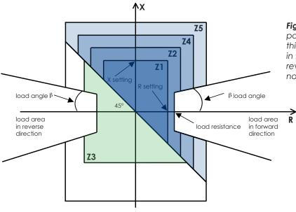
**Figure 2.** The distance protection polygonal characteristics. In this example zone 1 & 2 & 4 are in forward direction, zone 3 is in reverse direction and zone 5 is non-directional.
